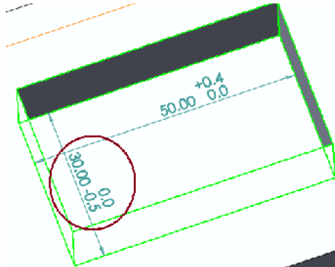
Illustrative Example of Pocket Feature that will be Machined to Mean
