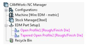
Inserted Vertical and Taper Open Profile Feature in Feature tree
